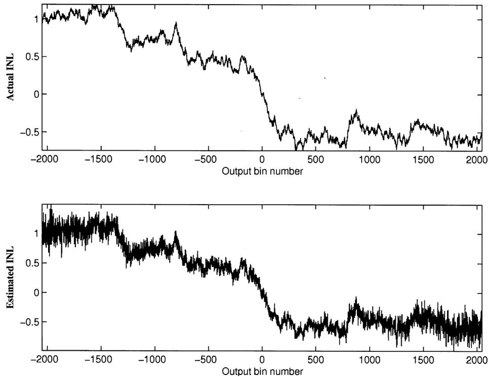
Fig. 9. ADC's modeled (actual) and estimated INL.
